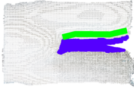
FIGURE 3.6: Leg cluster with detected RoI in purple and US trajectory in green.
