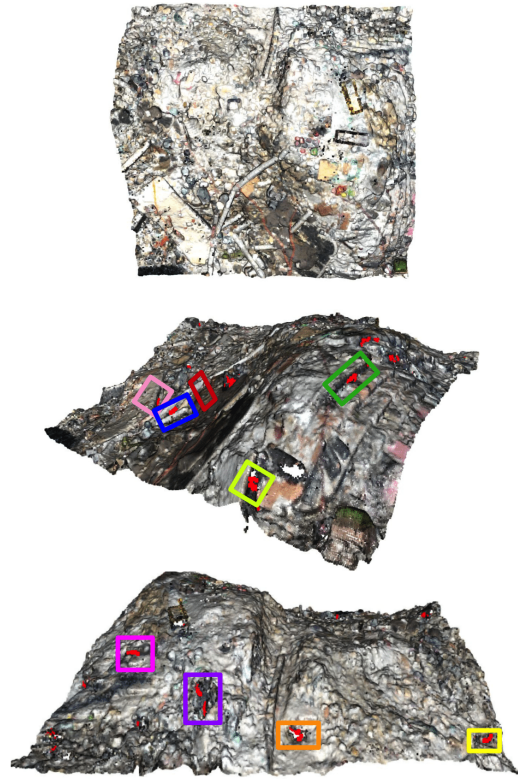
Fig. 4. Top: Point cloud from day 1 bounded by user-defined crop. Bottom: Detected candidate void regions (true and false positives) overlayed on the point cloud.
