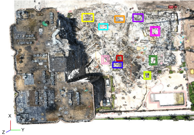
Fig. 3. Annotated regions corresponding to voids located in the collapse scene by experts. (Naturally occurring voids shown in double boundaries and voids created by excavation shown in single boundaries)
